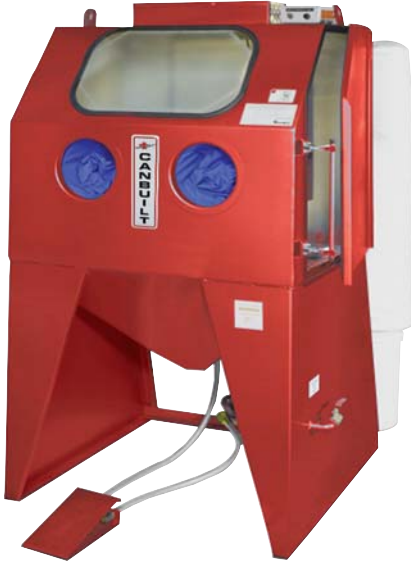
Model # BC-3MR Front View Recommended Media: Glass bead and Aluminium Oxide SAND NOT RECOMMENDED
